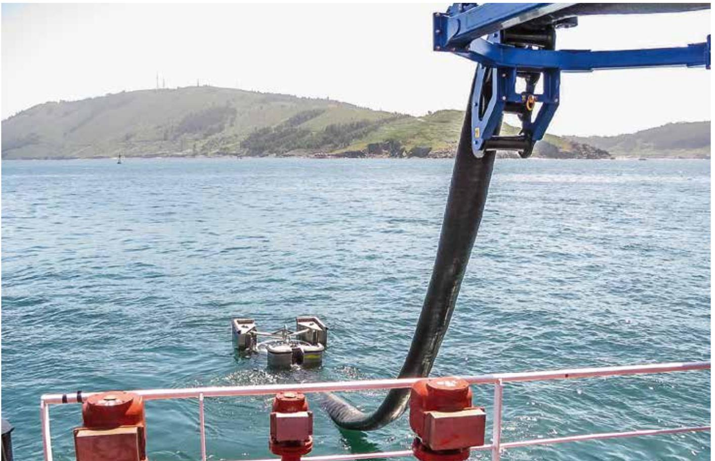
The remarkable thing about the oil recovery hoses is that they are inside a floating material, the outer surface of which is fortified to stand the hard weather conditions, oil as well as wear and tear. Also, the solution comes equipped with all components needed in recovery and oil transfer. Thanks to the telescopic extension arm, the hosing or collector are operable during emergency drainage by one person only, as well.
