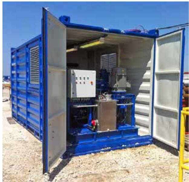
*No larger than this: PMC's compact cyclone reservoir can be seen in the middle of the opening. The image shows a pump aggregate mounted in a container. The reservoir holds just 120 litres but serves a system mounted with two 200 kW electric motors that each drive an Eaton Hydrokraft TVW-250. The transmission pumps each have an Eaton wing pump VMQ3525 as feed pumps and for supplying pilot oil. A Kawasaki K3VL80 is used as a working pump.*
