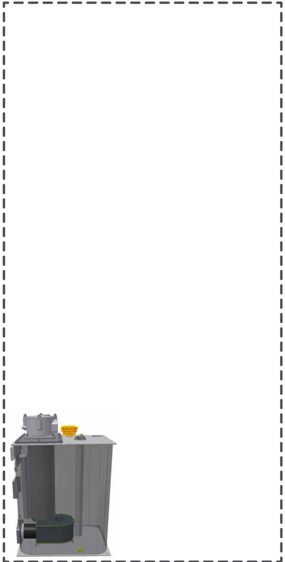
*Up to 90 % of the space (sometimes more) is left over when you replace a traditional hydraulic reservoir with the cyclone reservoir from PMC Group. Space that can be filled with new, competitive technology, or not be used at all – in that case, the compact reservoir reduces the total weight.*
