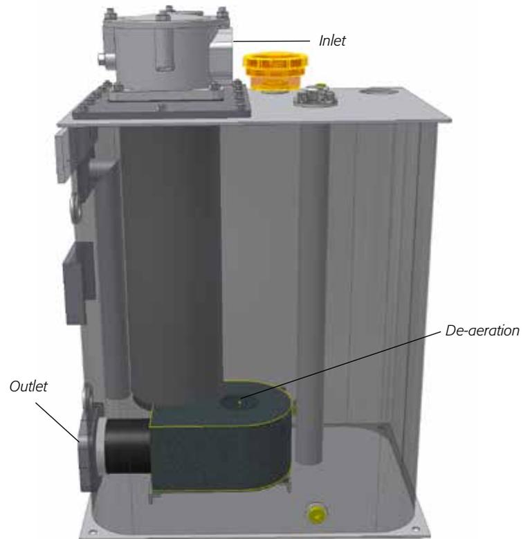
*In a cyclone insert, hydraulic fluid flows at high speed from the system's return line along the wall of the insert. In the resulting rotating airflow, the air is separated from the fluid due to its lower density. This insert is dimensioned for a return flow of up to 650 l/min. The size is approx. 250x130x185 mm. The insert is robust and of simple design – it does not have any moving parts other than a spring so is therefore very reliable.*
